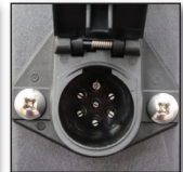
7-Way Round Pin Connection
