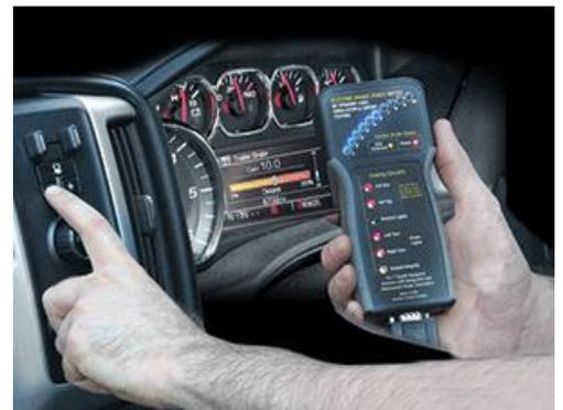
**#3: Some manufacturers use trailer detection technology on circuits other than the electric brake circuit**, such as 12V aux, left/right turn signals, etc. To verify proper operation and troubleshoot problems, you need the right tools to activate these circuits.
