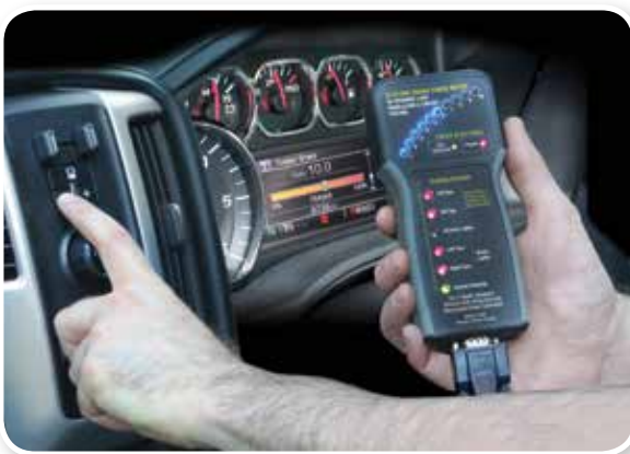
Real-Time Brake Force Output Gain and Timing
