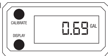
Fig. 3: Check reading after container is filled.
