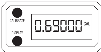
Fig. 4: In calibration mode enter the value read previously.
