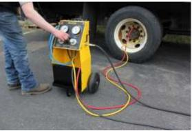
The **Mobile Tire Pressure Equalizer** is also optimized for adverse weather conditions with the recently upgraded design. It is mounted on a powder-coated steel body with pneumatic tires and features wheel-specific,color-coded hoses with corresponding panel indicators and convenient hose hangers. Simple to hook up, easy-to-use and with accurate and consistent results, the **Mobile Tire Pressure Equalizer**, made in the USA, is a professional solution for the tire service providers.
