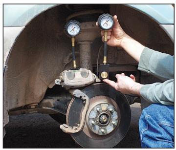
For 20 years the Disc Brake System Analyzer has been a critical tool for brake diagnostics.
